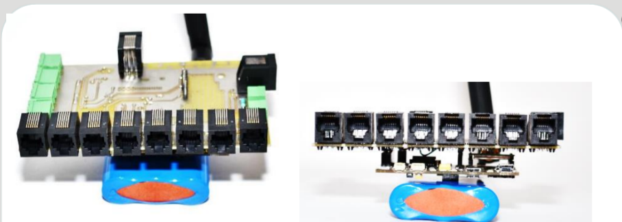
The custom board on top of a battery and a Wasmote from Libelium.
